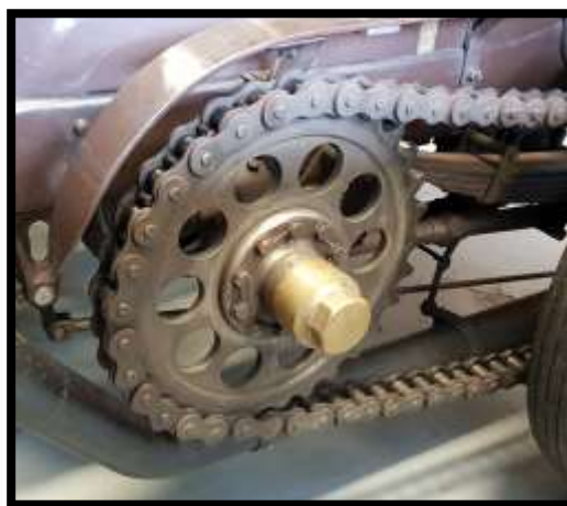
Above; The MAB is a big car. Below; V12 aero engine; massive drive sprocket and chain to get the power to the skinny wheels.
