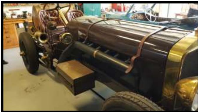
Above; The MAB is a big car. Below; V12 aero engine; massive drive sprocket and chain to get the power to the skinny wheels.
