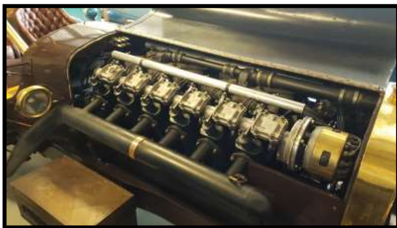
Above; The MAB is a big car. Below; V12 aero engine; massive drive sprocket and chain to get the power to the skinny wheels.
