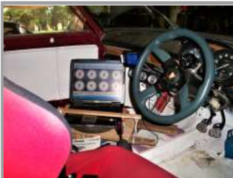
Laptop lashed to a frame for on track auto fuel mapping.
