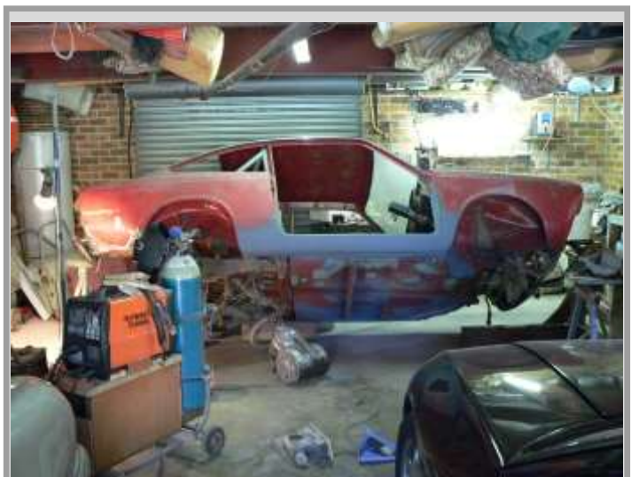
I built a simple rotisserie repair the rust in all the usual places. This is a very useful tool for working on a car body for repairs, modifications and restorations.
