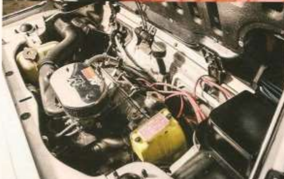
Clockwise from top left: the anticlockwise tacho runs to 8000rpm; red leather trim isn't for the shy and retiring; underbonnet tweaks include a K&N filter and electronic ignition; Nuccio Bertone nameplate proudly sits beneath the glovebox
