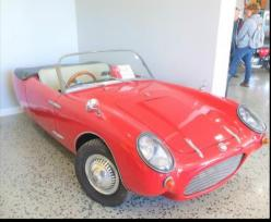
A Berkeley T6o three wheel sports car from England; front wheel drive powered by a 328 cc air cooled twin cylinder engine through a 4 speed gearbox.
