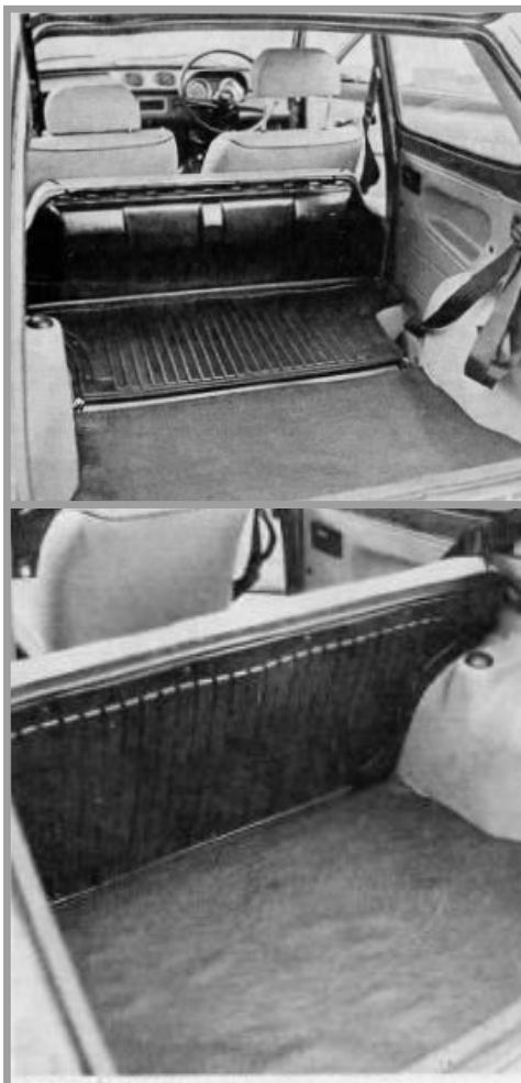
Comparison photos show the amount of space available with the rear seat squab raised and lowered. It's a pity that FIAT does not offer a Renault/VW style rear shelf to hide the contents of the boot, but pricing considerations precluded its inclusion.
