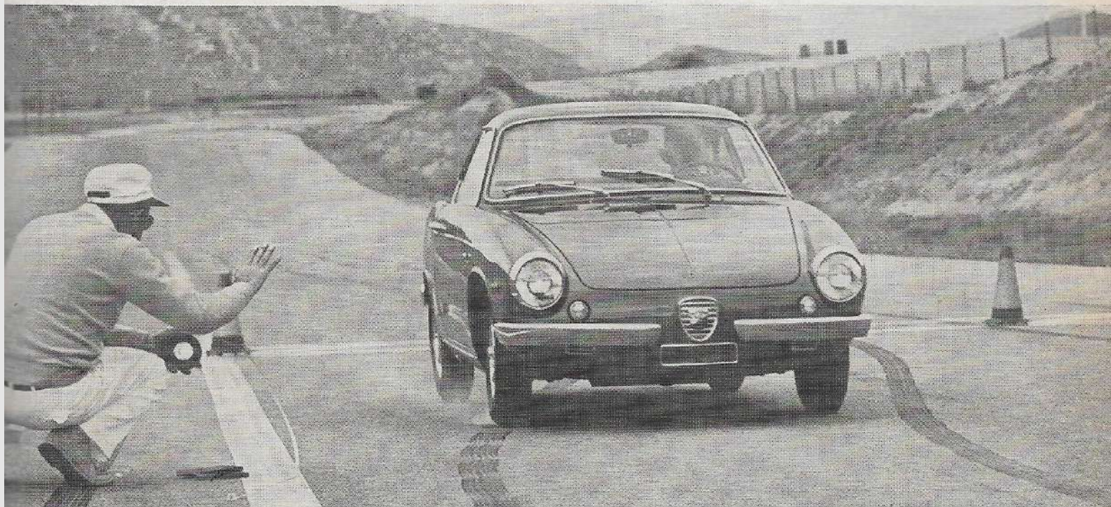
ALL-OUT PANIC STOPS FROM 60 MPH BROUGHT THE CAR TO A TIRE-RIPPING 140-FOOT STOP WITH NO SWERVE OR LOSS OF STABILITY.
