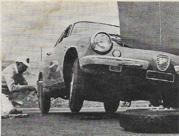
Single jack-point serves each side; car is simple to lift. Basic tool kit contains screwdriver, wrenches and jack.
